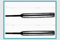
Measures diameter, cone angle and wall thickness of balloon
